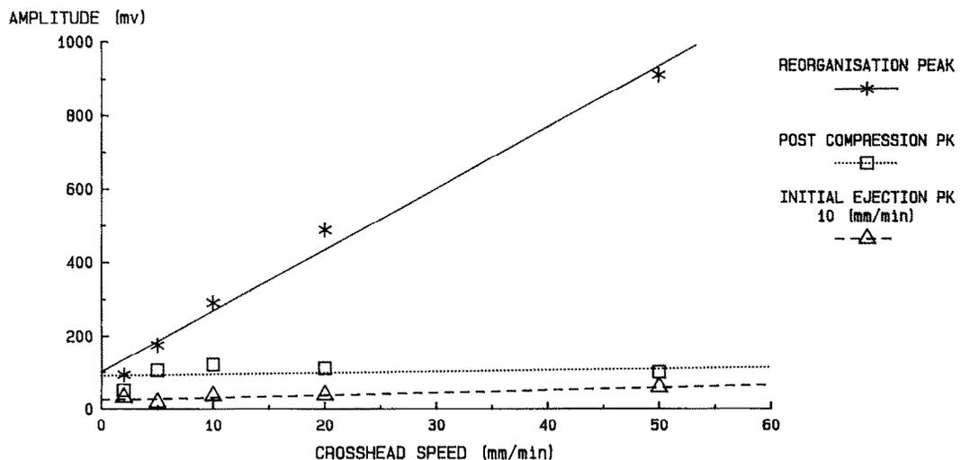
Fig. 10. The effect of compression speed on the amplitude of the acoustic emissions from sodium chloride, 200–250  $\mu\text{m}$ .
