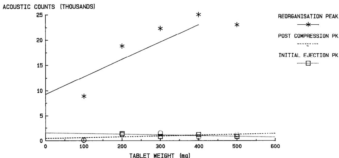
Fig. 6. The effect of tablet weight on the A.E. from sodium chloride, 200–250  $\mu$ m, during compression and ejection.
