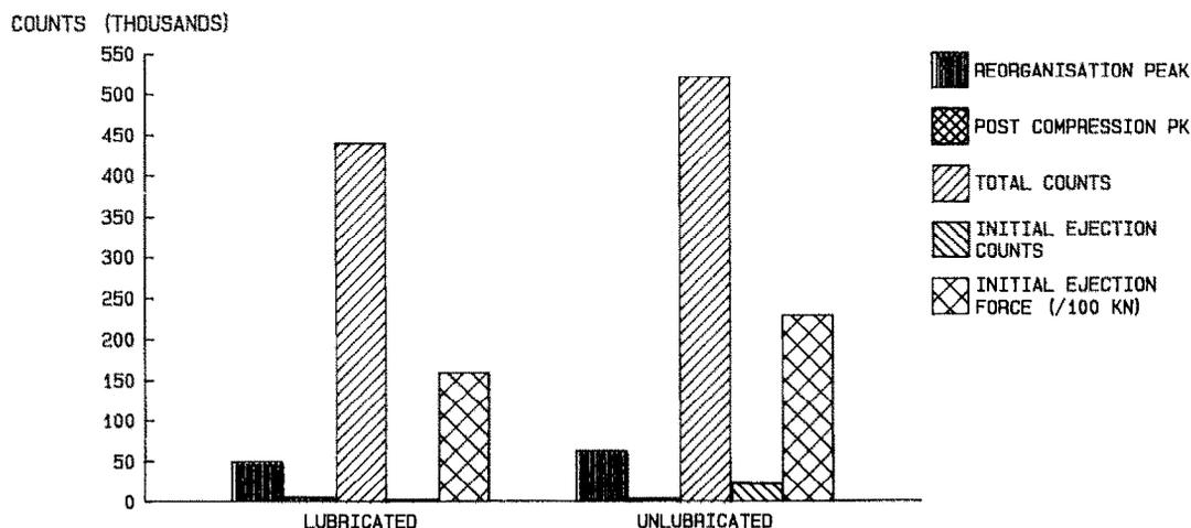
Fig. 2. The effect of lubrication on the A.E. from sodium chloride, 200-250  $\mu$ m.
