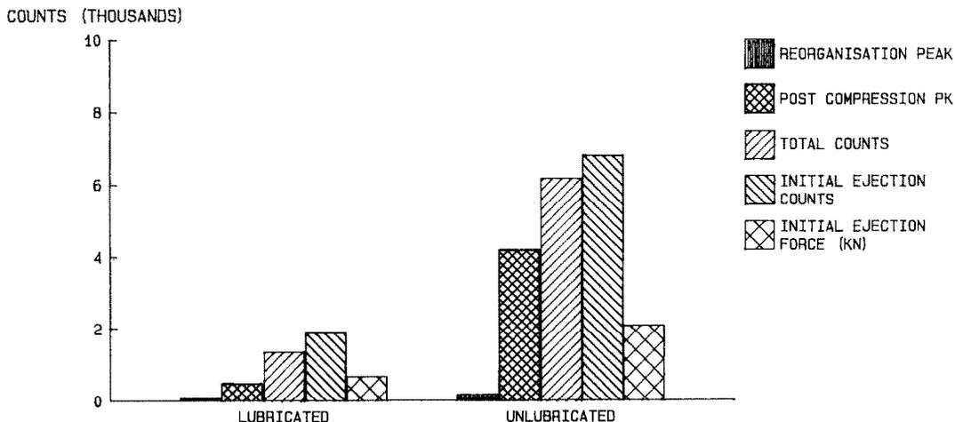
Fig. 4. The effect of lubrication on the A.E. from: Zeparox, 32-63  $\mu\text{m}$ .
