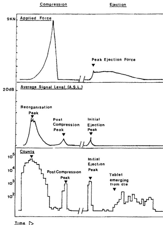
Fig. 1. Acoustic and force profiles of sodium chloride, 200-250  $\mu\text{m}$ . All profiles to the same time base.
