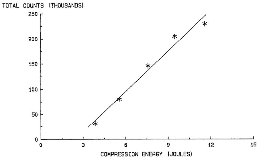
Fig. 8. The effect of compression energy on the total acoustic counts measured during compression of sodium chloride, 200–250  $\mu$ m.
