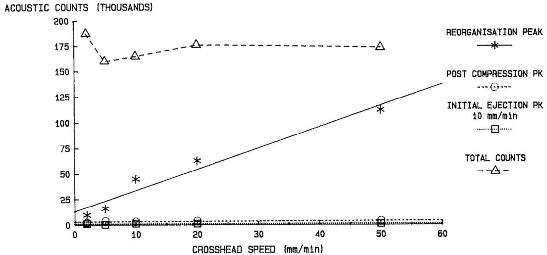
Fig. 9. The effect of compression speed on the A.E. from sodium chloride, 200–250  $\mu\text{m}$ . Ejection speed maintained at 10 mm/min.
