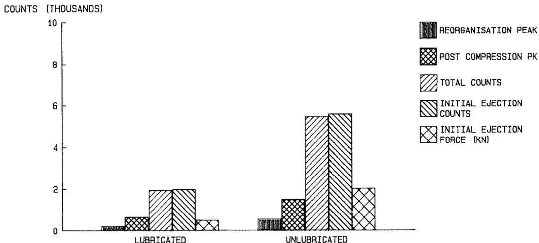
Fig. 3. The effect of lubrication on the A.E. from lactose monohydrate.
