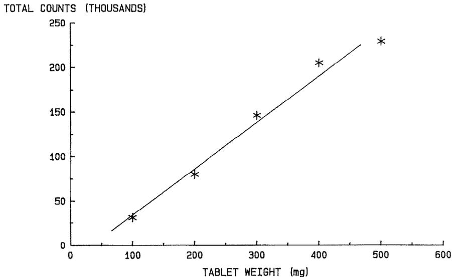
Fig. 7. The effect of tablet weight on the total acoustic counts measured during compression of sodium chloride, 200–250  $\mu$ m.
