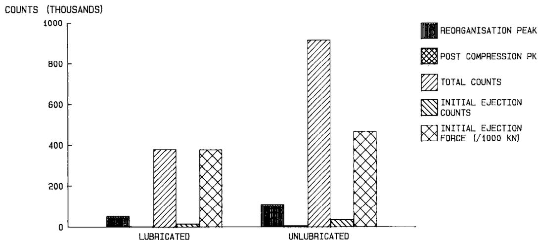
Fig. 5. The effect of lubrication on the A.E. from paracetamol.
